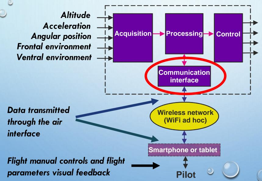
Process consisting in moving the drone in accordance with the flight controls transmitted by the pilot
