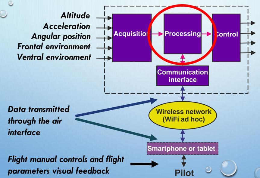
Process consisting in moving the drone in accordance with the flight controls transmitted by the pilot
