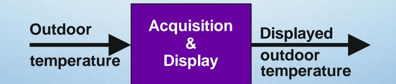
Input information : outdoor temperature (physical parameter) Output information : displayed value of the temperature (in °C)
